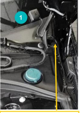
Use a tie-wrap to secure the cable
