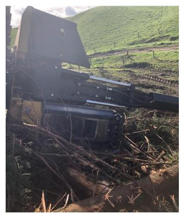
An incident occurred where a felling machine tipped over and the emergency exit could not be used.
