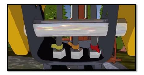
With the head attached the machine operator started work about 8am. But by 9am the machine broke down again. A sensor joint had blown because of the incorrectly fitted hoses. The machine operator went to find a replacement part then returned at 1.30pm and began to fit the new part. It wasn't until 3.30pm that he was able to get back to work.
