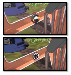
• Redesign the hoses to be one-way installed: Fitting the hydraulic hoses incorrectly is a very common problem. Redesigning the hoses to be one-way installed would be simple and would prevent a tremendous amount of damage being done to machines across the industry.
