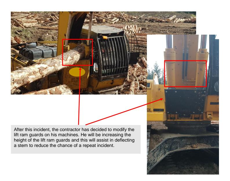
This incident resulted in machine damage exceeding \$50k, but thankfully the operator walked away with a bruised arm. Operator protective structures are effective if they are certified and inspected annually. Ensure that protective structures are re-certified after major structural damage.
