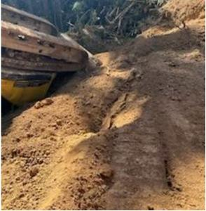
An incident occurred where an earthmoving excavator tipped over while developing a skid.
