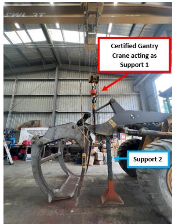
Wheel loader being worked on in the workshop. 2 support systems in place.
