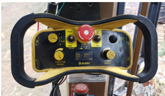
Remote control systems that incorporate safety redundancies.
