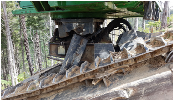
Extended (>50mm) single grouser track shoes for tracked machines and chains or bands for rubber tyred machines.
