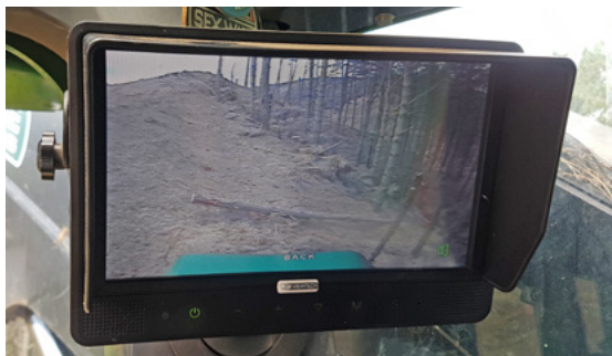
Camera display of obstructed view areas for the operator including winch.
