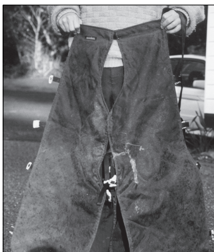
Cuts to chainsaw chaps make them unsafe
