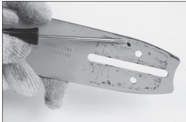
Clean the guide bar lubrication holes
