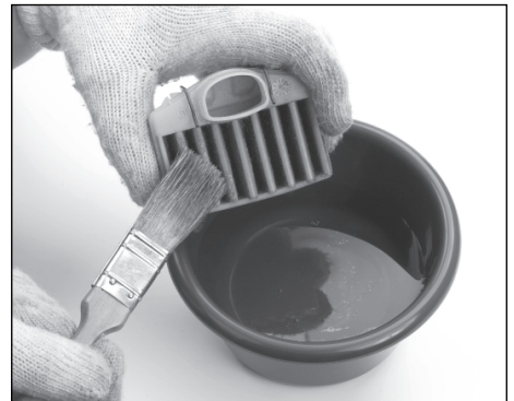
Use a brush to clean the air filter
