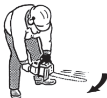
Chain brake operated by inertia
