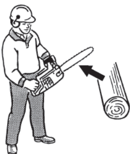
Chain brake operated by hand guard
