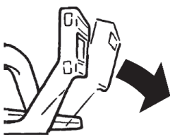
Chain brake operated by hand guard
