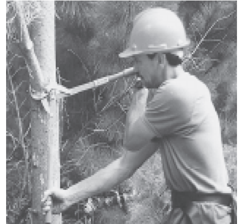
Place the blade against the tree and squeeze the blade into the branch.
