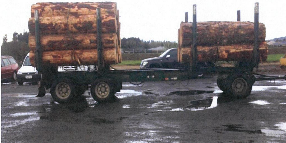
Figure 20. 3.1 metre on a 3 axle trailer – Photo shows logs almost over on rear packet technically, but well loaded topped and tailed and correctly crowned.
