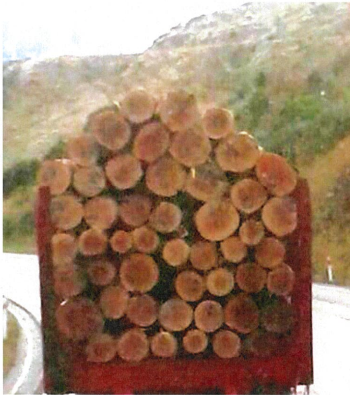
Figure 30. Over height but well crowned for chain contact however absolutely not acceptable, not even if load is light. Must be within the volumetric capacity of the bolsters as per Figure 28.
