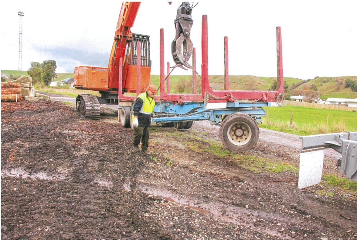
Figure 9. Pull drawbar around with handle. Note back wheels can be on ground or whole trailer suspended.
