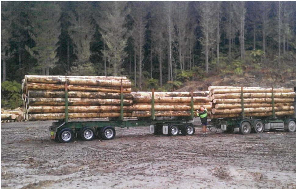
Figure 26. What is wrong with this load? Normal rules still apply even for off highway. Weight may increase a little but is still limited by the vehicle certification (GVM)
