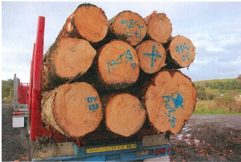
Figure 15. Load Foundation tight, 2 nd row tight, top row crowned for chains to touch all logs. Awesome
