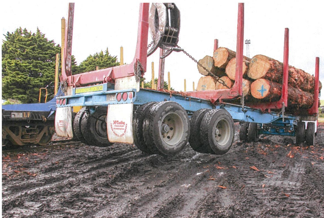
Figure 12. ABSOLUTE NO - NO loading the front packet then swinging trailer around by the lifting chain. This bad practice results in premature chain wear and possible failure. Side loading the front packet is OK when loader reach is compromised but the trailer must be pulled ahead by the truck to load the rear packet.
