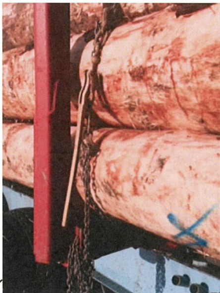
Base tight 2 nd layer tight and top crowned. Secured easily and properly. No problems in transit. ✓✓✓ Next Load.
