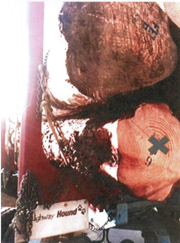
Bottom layer not touching bolster so not tight 2 nd log not touching. Relying on the chain but very hard to get and keep tight.
