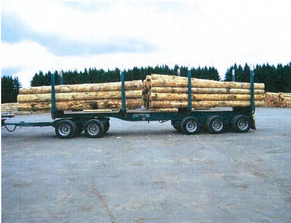
Figure 19. The same load but double bunked. Note how much lower and longer it is. Result is much better stability.
