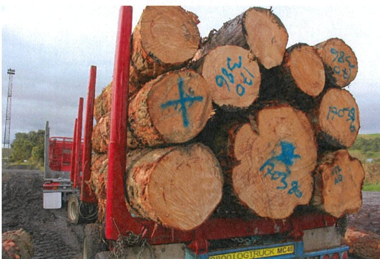
Figure 14. Load Foundation OK and load well rounded. Note big log on the first layer.
