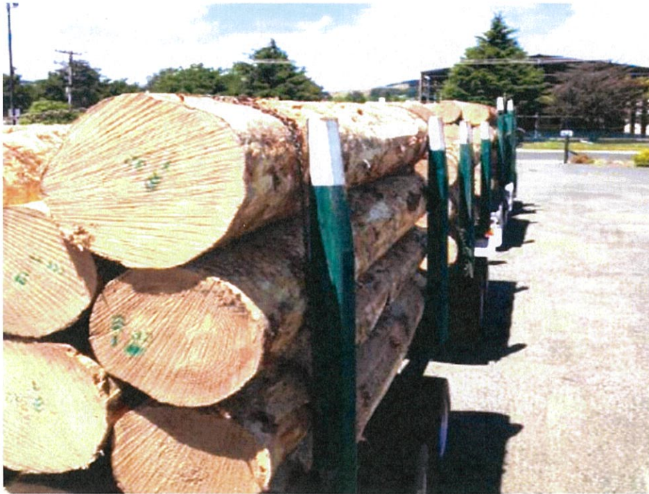
Figure 17. Barely over height but it is over height according to the ACOP
