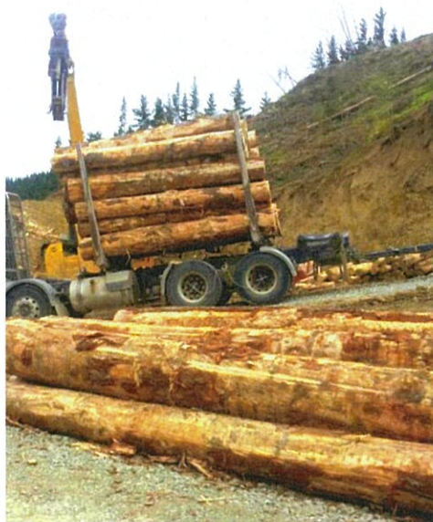
Figure 16. Logs sliding forward due to truck being loaded on a slope.
