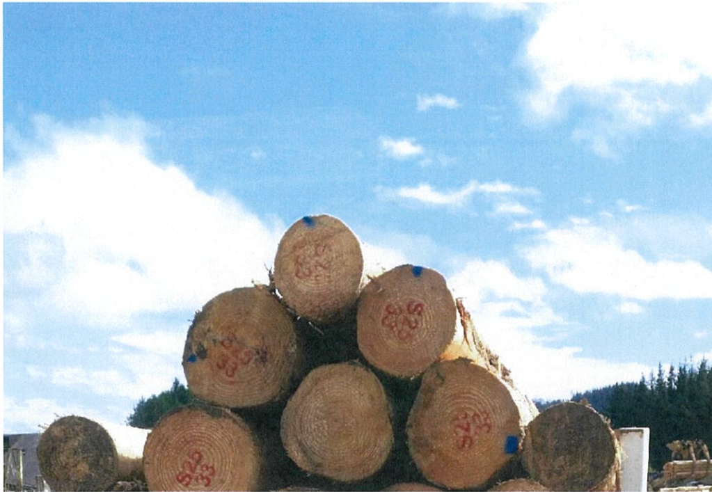
Figure 28. Poor crowning. Logs over top of bolsters not supported by 2/3rds of log next to them. Outside log technically too high.
