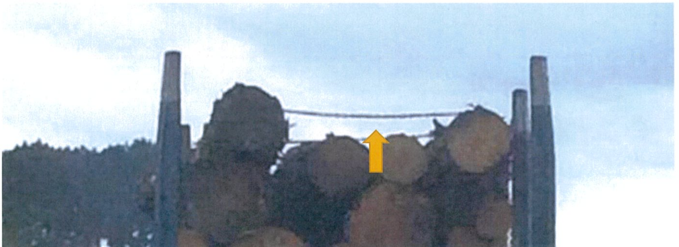
Figure 23. Poor crowning. Logs in middle have no chains on them.
