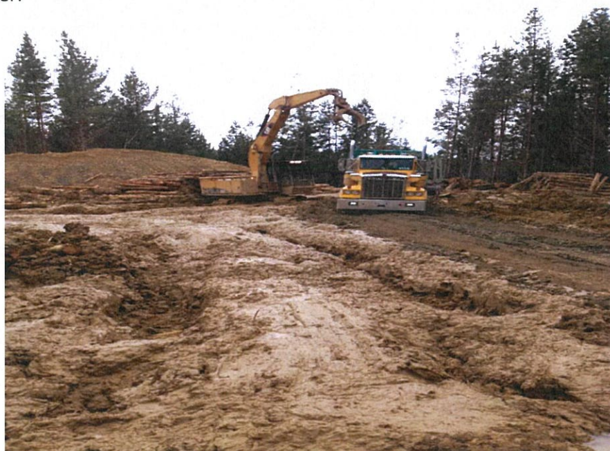
Figure 21. Muddy landings. In the dark a major cause of injury. Trucks should move away to a better place to chain up if it is safer up to 100 metres.
