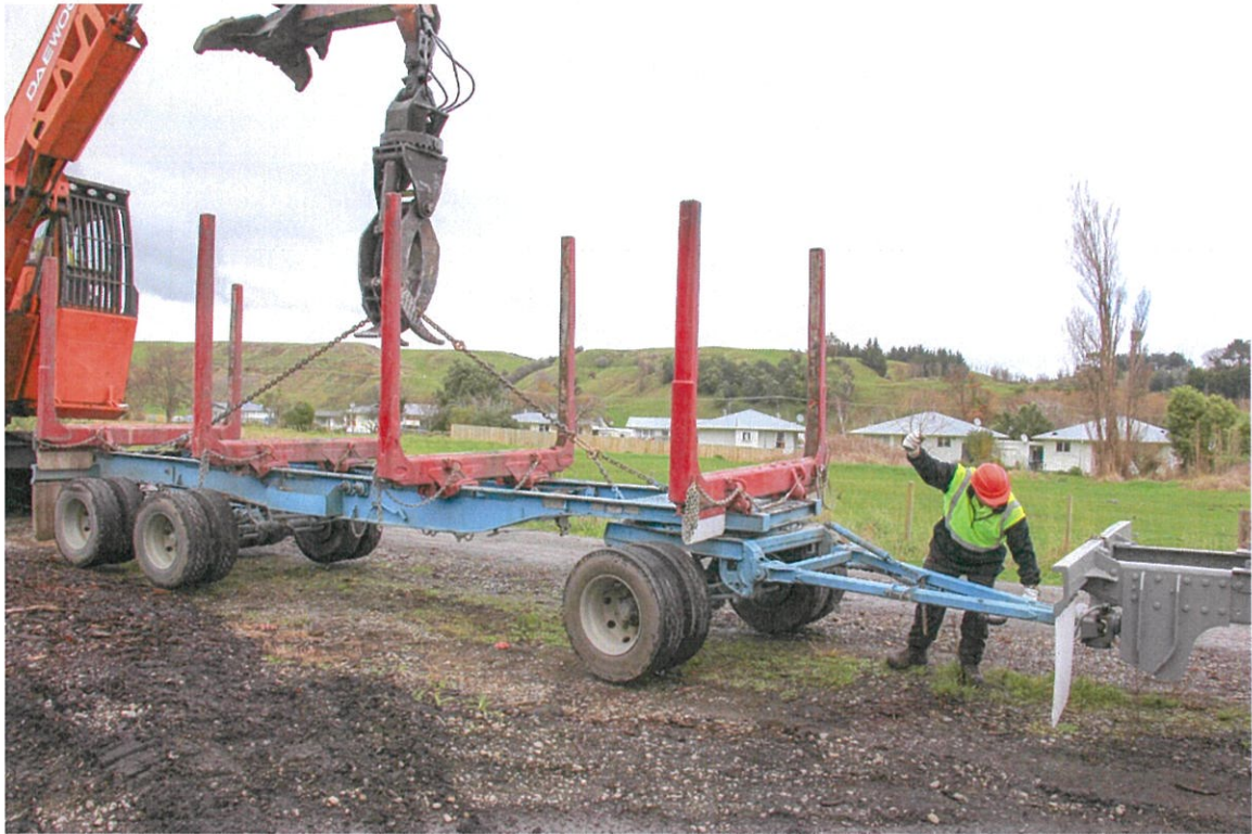
Figure 10. Hands well clear of any steel contact or jamming. Indicate to Loader Operator what you require, ahead – back – etc.
