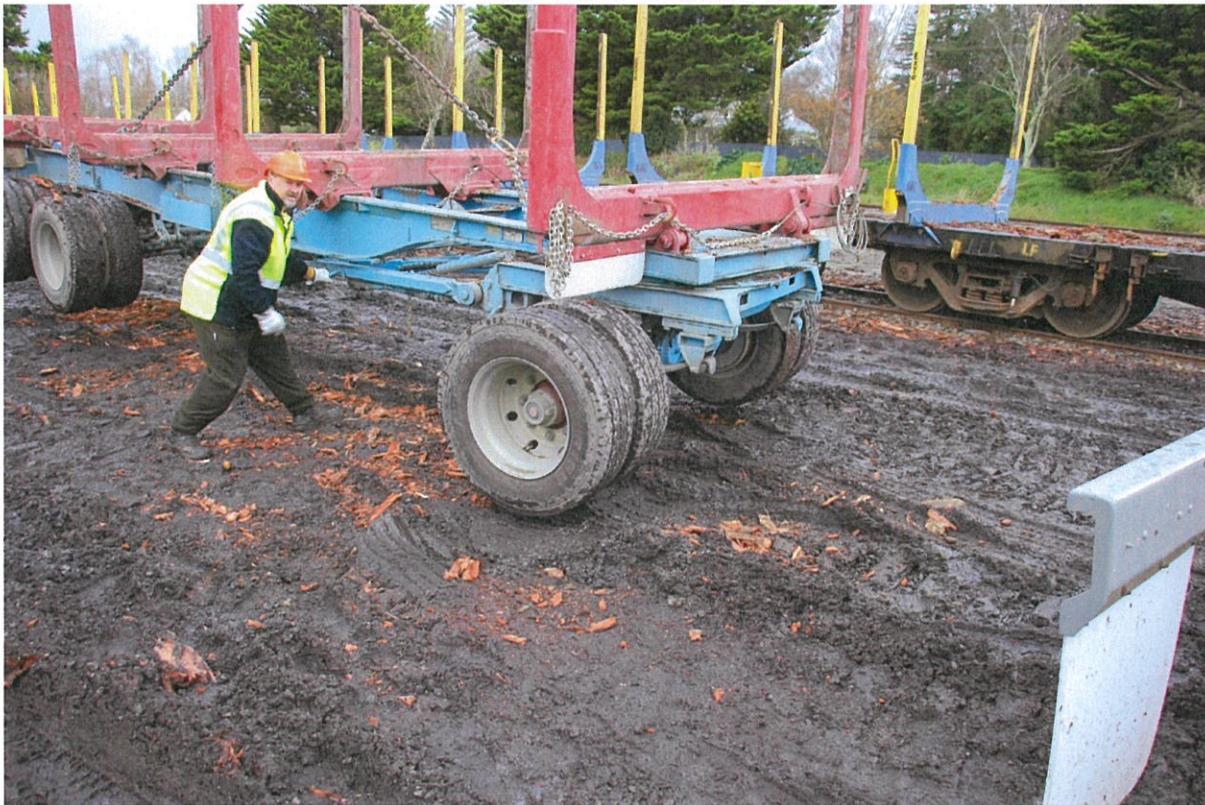
Figure 8. Unhook drawbar and turn. Note height from ground nothing other than an arm under the trailer.
