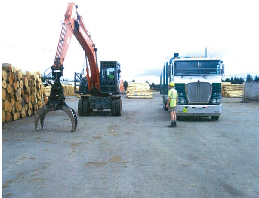
Figure 2. Loader parked with door facing the door of the truck and grapple lowered. Loader drivers should look to park similar to this way whenever the truck driver is in the loading zone.
