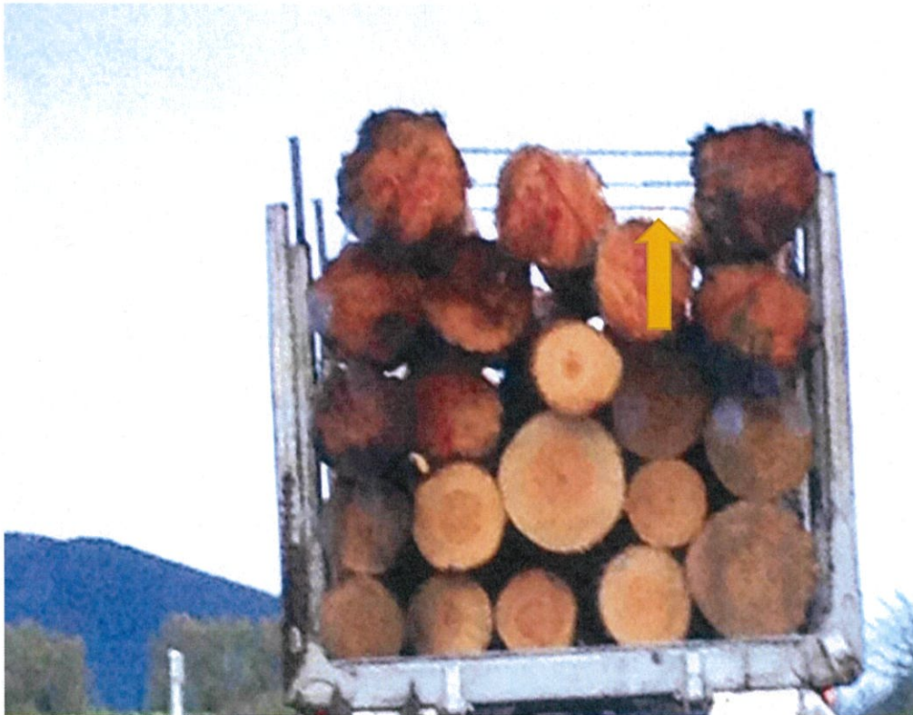
Figure 22. Poor rounding of the load. Chains should touch all top logs ensuring they are locked into one another or pulling down on the next log.
