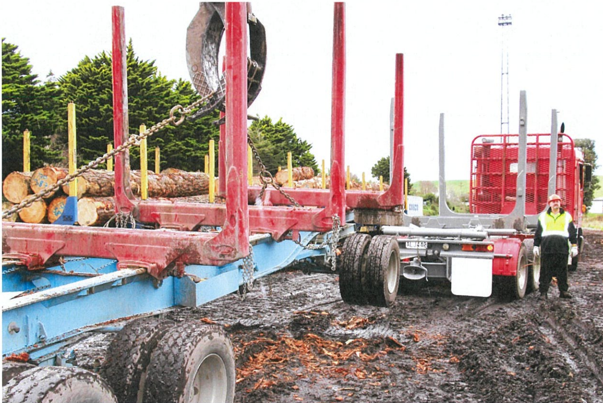
Figure 6. Wait until loader operator gives OK by signal or radio if using one.
