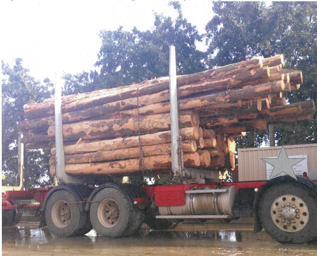
Figure 29. Top heavy loading. Longer logs should be on the bottom.
