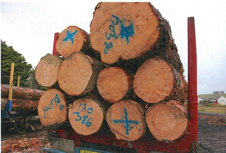
Figure 13. Poor loading. Big log on top r SRT and 2 nd layer not touching bolsters but rounded enough.
