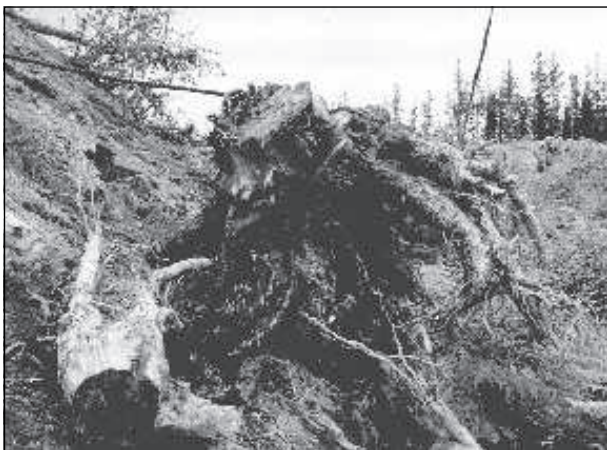
Do not use old rotting stumps. This 2-year-old stump failed, causing a tower to overturn
