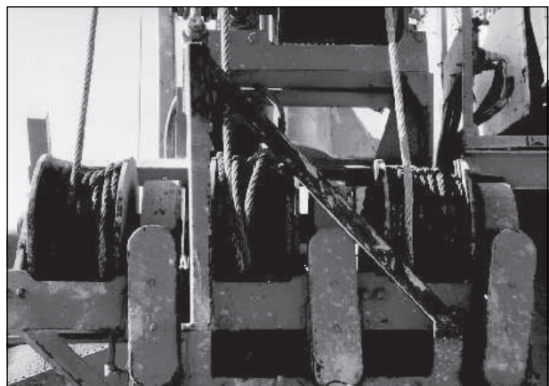
Avoid poorly fleeted drums - these may result in poor guyline balance
