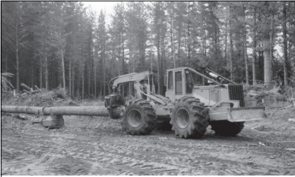
A grapple skidder pulling stems straight through a delimber
