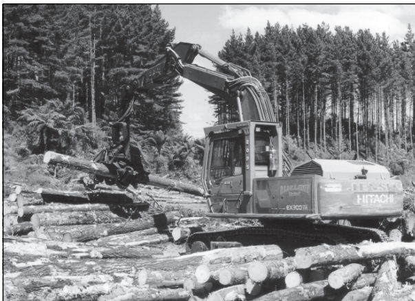
Log-making with a mechanised processor. Stems are fed right to left to give the operator a better view of log characteristics.
