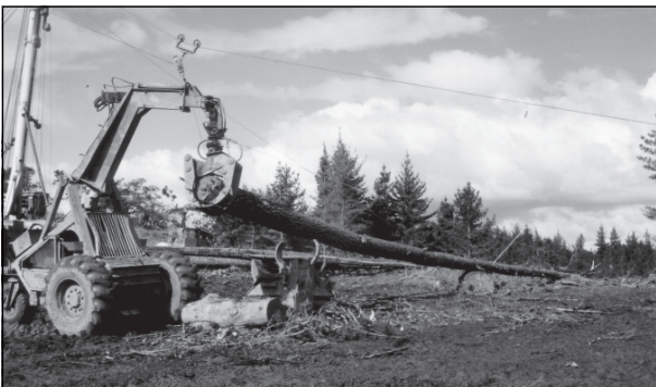
Using short logs to support the stem and help anchor the delimber
