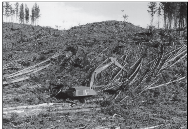
Machine delimiting and bunching stems off a slope
