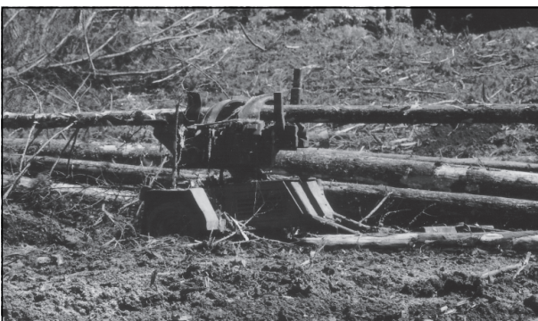
Position the delimber on stable ground
