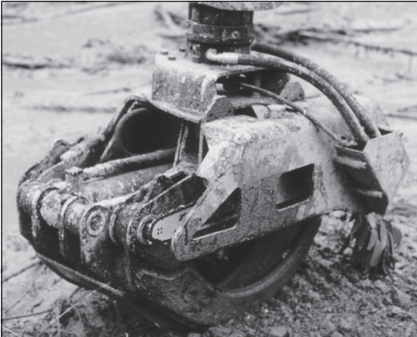
A Waratah cut-off saw attached to the front of the grapple
