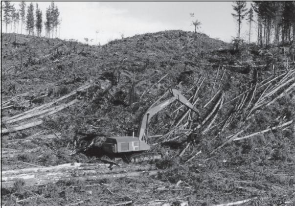
A stem being processed through a Waratah harvester/processor head
