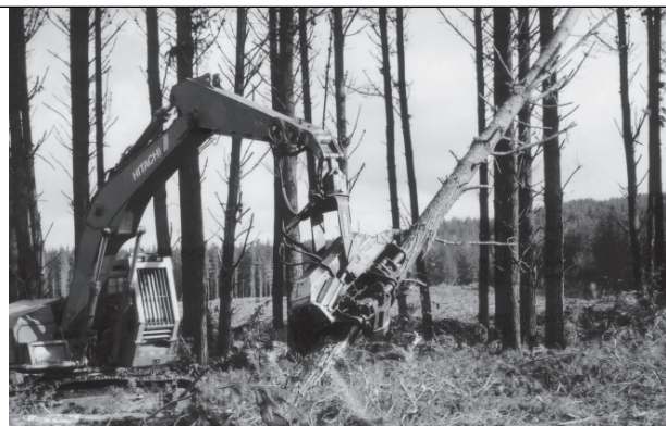
As the tree begins to fall, lift the butt and slew the tree away from the intended direction of fall
