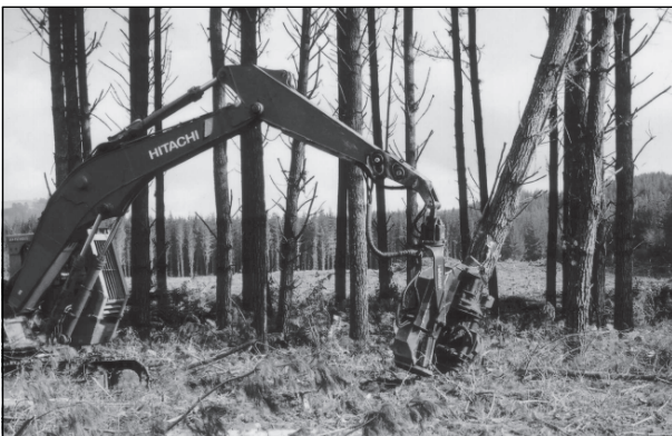
As the tree begins to fall, lift the butt and slew the tree away from the intended direction of fall
