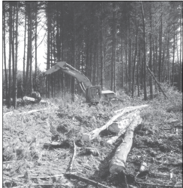
A feller-director machine slewing the felled trees on to bunches down either side of the machine. In this case the trees are being delimited on to the bunch.
