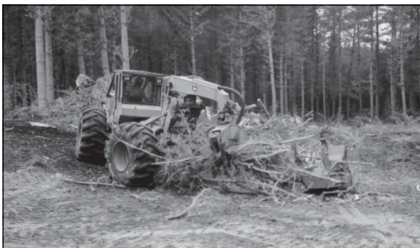
Clear debris from around the delimeter when it starts to hinder the operation
