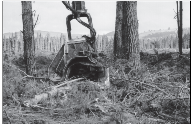
Clearing slash and understorey from the base of the tree
