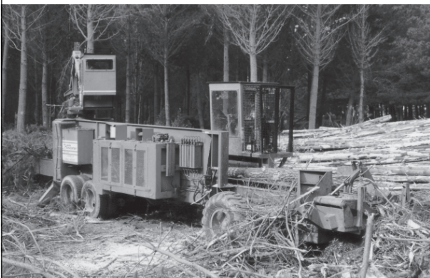
A Hahn Tree Harvester. The remote loading grapple is on the left. The operator sits in the cab in the middle.
