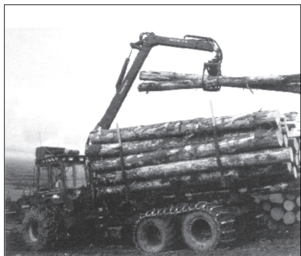
A forwarder with band tracks fitted to the rear bogies
