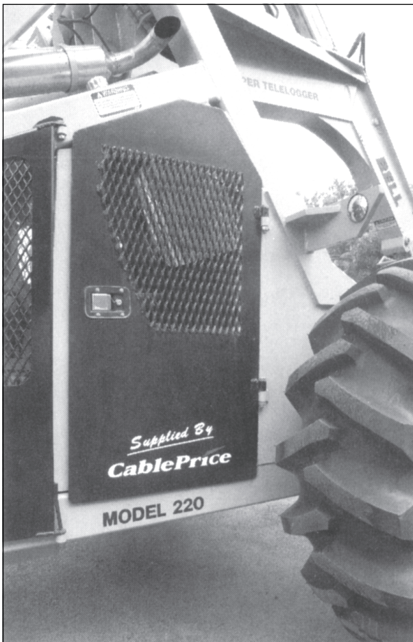
Ensure that doors are closed as these form part of the OPS
