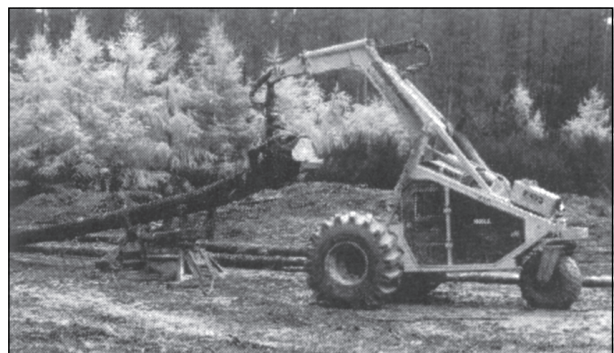
A Bell loader pulling a stem through a static delimber
