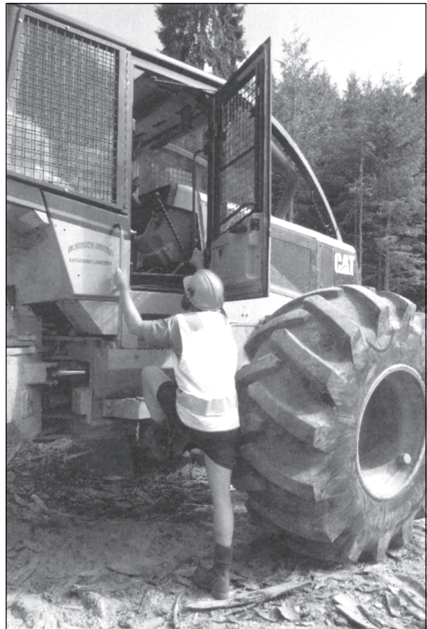
Use appropriate hand rails and steps
