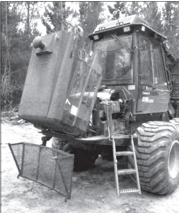
Check and clean debris from the engine compartment
