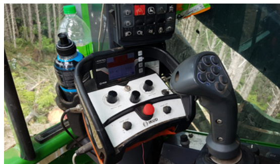
Prevent accidental operation of the Steep Slope Harvesting machine when the winch is in manual mode.
