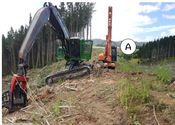
A Excavator is back far enough to allow the felling machine to be on the rope as it moves over the edge
