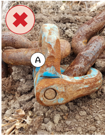
A Hammerlock worn by rubbing against machine. This happens when going to flatter slopes below steeper ones
