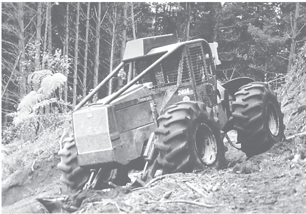
Machine positioned for hook-on (note blade in the down position)
