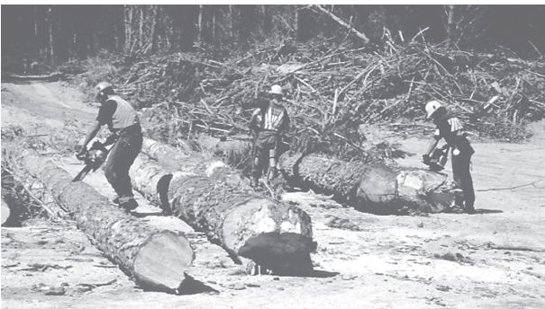
Stems laid out for manual processing
