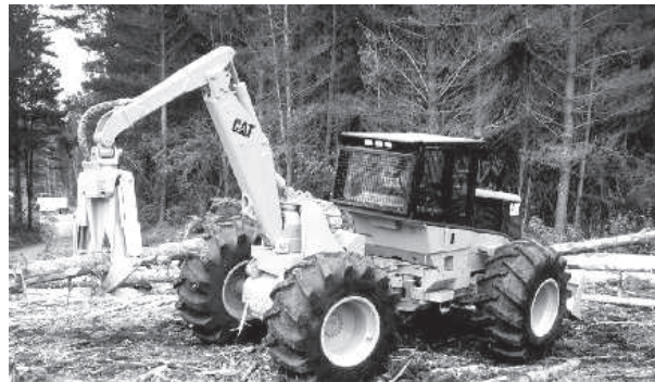
Swing-boom grapple skidder
