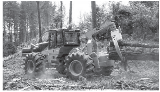
Conventional grapple skidder
