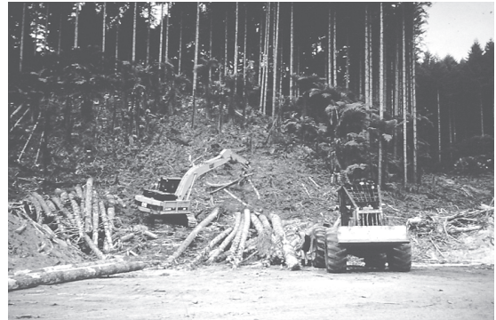
Stems bunched for the skidder
