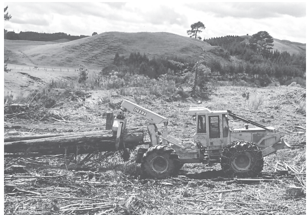
Travelling loaded, blade up and butts off the ground
