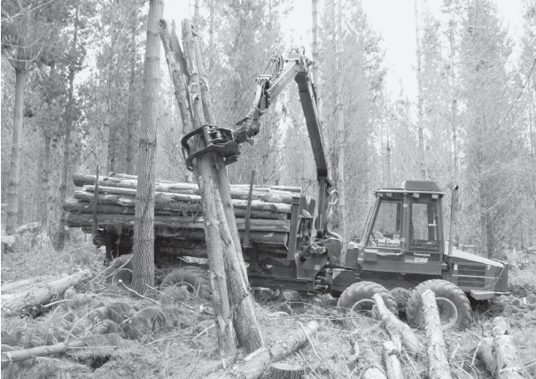
Aligning logs by “pencilling”
