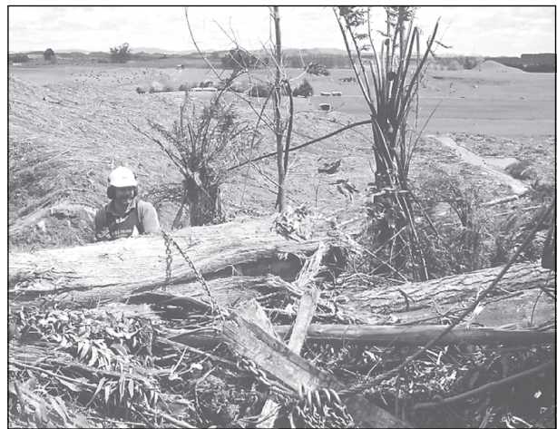
Pass the strop over the stem, then back under to hook-on
