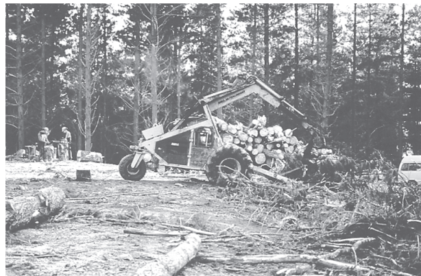
A Bell loader clearing slash from the work area
