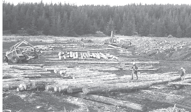
Separate work areas reduce machine hazards for manual workers
