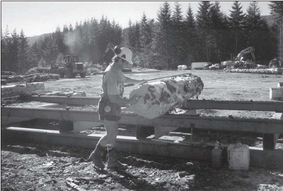
A skiddy carrying out quality control (QC) — checking logs for length and grade
