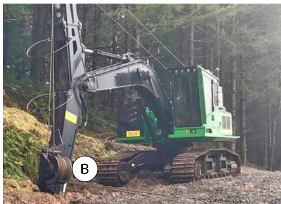
B Ensures the bucket is in strong natural soil or in hard ground on a track
