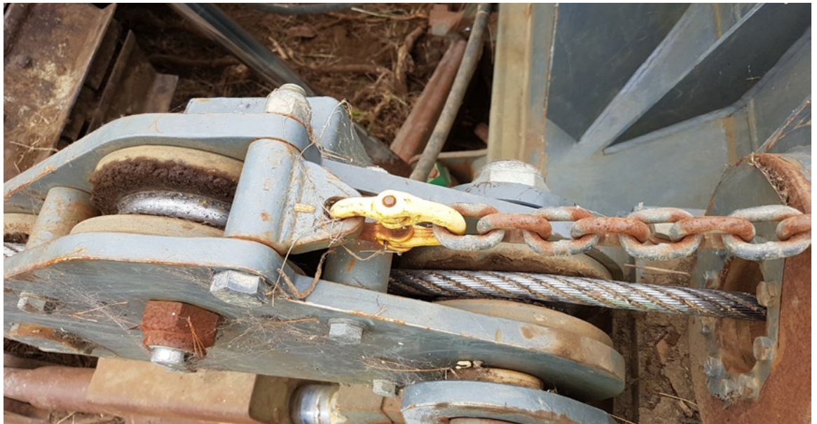
A three sheave deflection winch tension monitor system.
