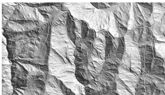
Old tracks can easily be seen with LiDAR, even with the trees still standing.
