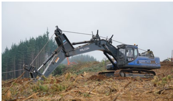
Left: the single winch DC Equipment's Falcon winch assist. Right: The twin drum EMS Tractionline. Below left: the Remote Operated Bulldozer (ROB). Below right: Eco-Forst T-WINCH 10.2.
