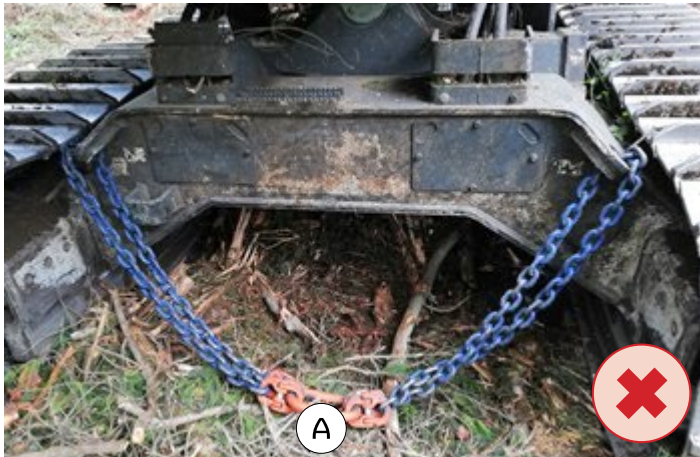
A Risk of extreme side loading of chain link
