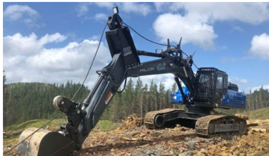
These are a few examples of commercial models available, top left: Eco-Forst T-WINCH 30.2. Top right: T Max. Below left: Electrical and Machinery Services (EMS) Tractionline and below right: DC Equipment's Falcon winch-assist.
