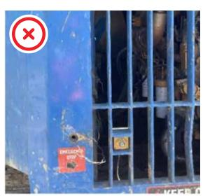
Engine guarding secured with a molly, not a bolt (tools required), as designed.
