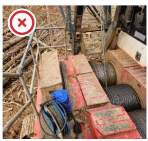
Right: The toolbox, hose, and 20-litre container location forces the operator towards a narrow walkway next to unguarded main winch ropes. Also, standing on top of the toolbox makes the guard rail below the required height.
