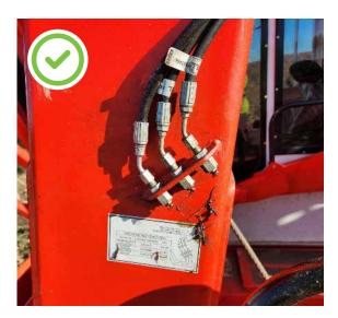
Tower grease points on the deck eliminate climbing or lowering the tower to grease.
