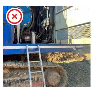
Although this is a latched and locked bay, the ladder (a good idea to improve access) does not have non-slip steps
