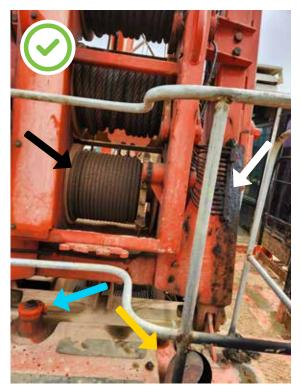
Post-manufacture railing and grease points reduce risk from heat (yellow arrow), trips and slips (blue), entanglement (black), and falls (white).
