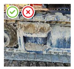
Excellent access steps choked with mud, now a hazard due to slipping and leg grating down the steps' serrated edges. The amount of mud indicates the risk is normalised.
