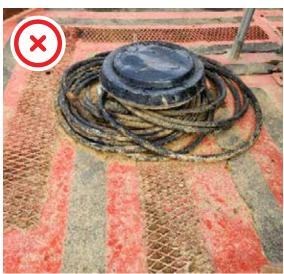
The walkway has protruding parts and hydraulic hoses coiled around it
