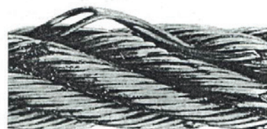
10. Wire fractures at the strand, or core interface, as distinct from 'crown' fractures, caused by failure of core support.
