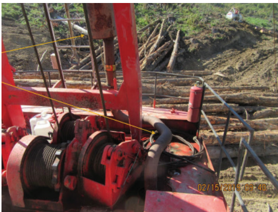
Unguarded potentially hot exhaust and muffler adjacent to access ladder.
