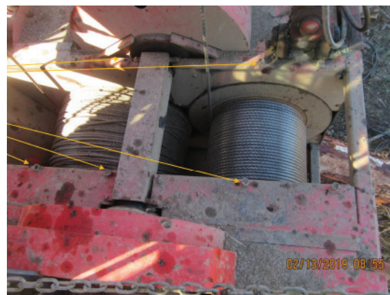
OEM handrails missing on a swing yarder winch set – original mounting points arrowed.
