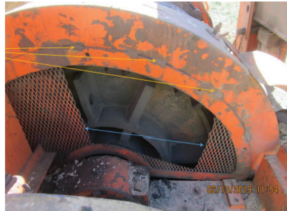
OEM guard (missing) had been replaced with the welded mesh shown after a toe amputation. Guard was not removeable "using tools", so has been cut out at some time to attach a new skyline.
