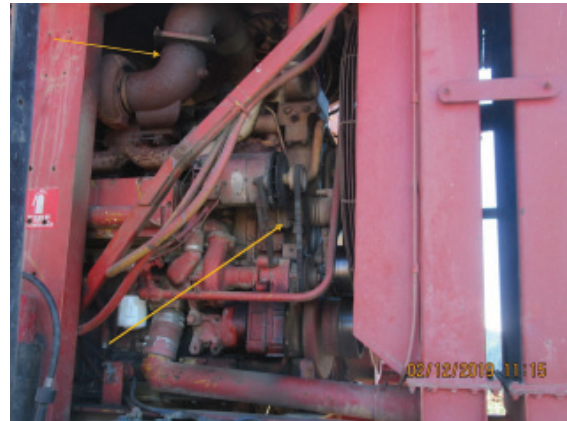
Entanglement risk from exposed belts and pulleys.
