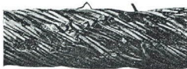
9. Typical wire fractures as a result of bend fatigue.
