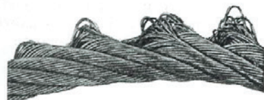
12. Strand core protrusion as a result of torsional unbalance created by 'drop ball' application. (i.e. shock loading).
