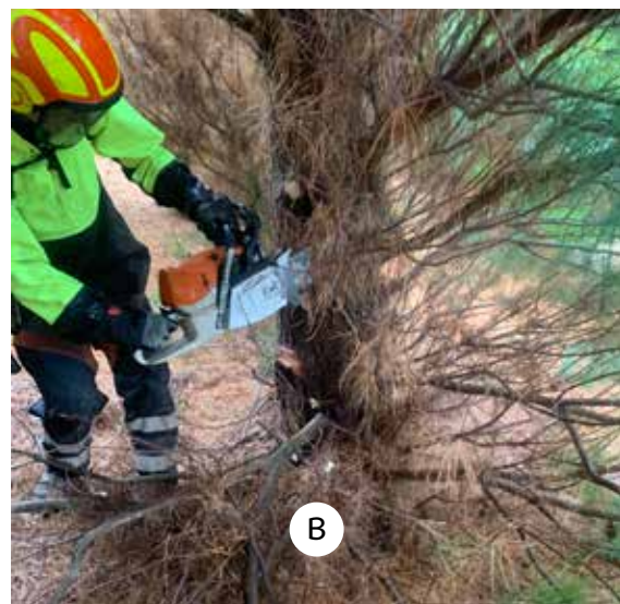
B Trim to the right (anticlockwise) to finish the tree.
