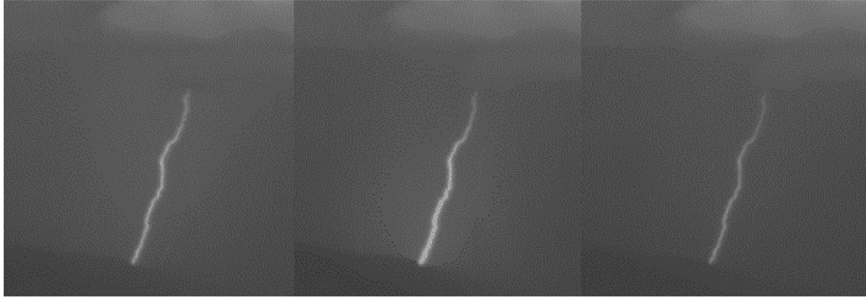
Fig. 2. Second (FI2), fifth (SU2) and seventh (SU2) stroke following the same channel to ground (from left to right).
