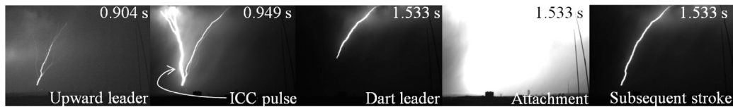
Fig. 4. The different processes in upward flashes caught with a high-speed camera.
