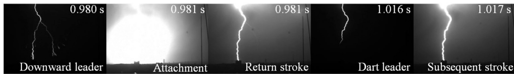
Fig. 3. The different processes in downward flashes caught with a high-speed camera.
